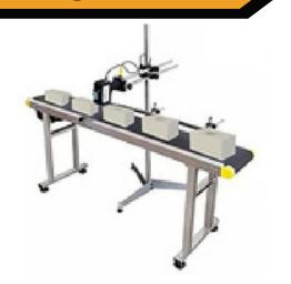
The batch number, batch code, or lot number must be displayed on the goods in accordance with local regulations. Batch coding machines added information to your product by stamping a mark or number onto the product's packaging or right onto the item itself.
