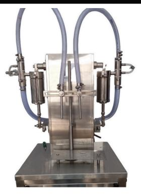
Semi-automatic filling machines are used in a variety of industries to put raw components into bottles and package them to make finished goods. Volumetric Syrings (cylinders) are used for the filling process, allowing the fill volume to be manually adjusted. Working on the volumetric principle, the small, adaptable Volumetric Bottle Liquid Filling Machine unit is housed in a body of beautifully matte-finished stainless steel.
